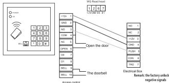
Note: Restore the factory settings (after the power cut OPEN and GND short together. Wait 3 seconds on the power to hear the initial success of Didi Didi 5 sound)
