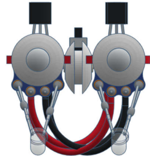
sensor cables crossed
