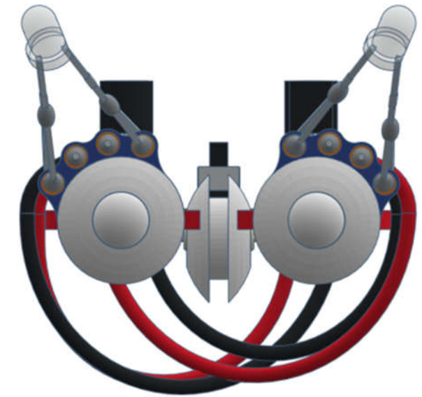
sensor cables crossed
