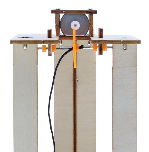
Finally, the cable is led through the elevator roof and knotted around one of the locking hooks.
