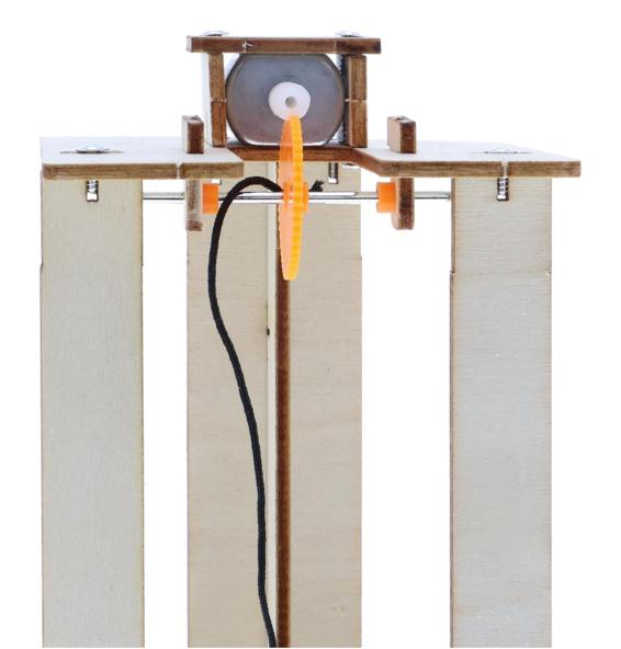
So that the cable thread remains secure in the thread holder, it is now fixed again from the other side with the orange spacers.
