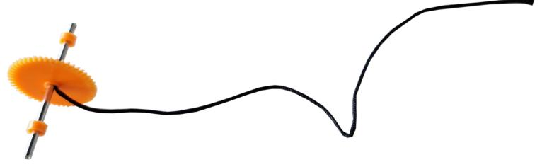
Now insert the cable thread into the thread holder so that the gear is in contact with the thread of the motor.
