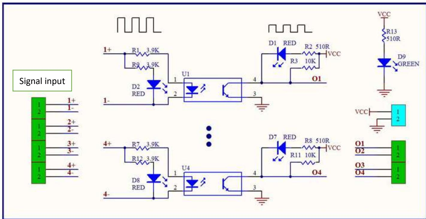
**Diagram of module wiring:** (Module power supply is equivalent to output signal voltage, Take "24V to 5V" as an example, and the signal conversion of other voltages are the same)
