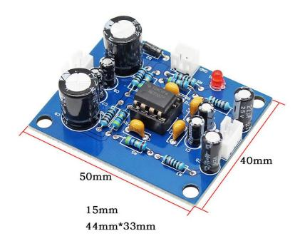
This microphone amplifier module is a high-quality solution for audio projects requiring reliable amplification and signal processing. Built around the NE5532 IC, it provides precise sound amplification, making it suitable for applications like voice recording, audio streaming, and DIY audio projects. With easy connections and stable components, the module is ideal for both beginners and professionals.
